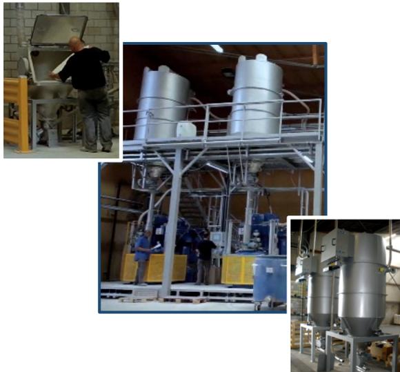
The installation is prepared to produce several t/h of finish product, working with two conveying lines installed in parallel. The products are sucked from different feeders, in function of the production order given by the supervision software. The powders are then dispensed into the final receiver.
